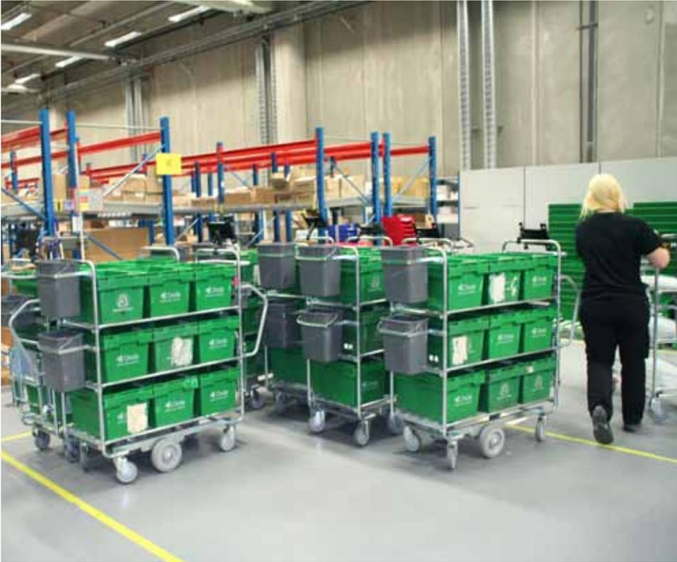
The trolley was designed in three versions with different picking options: six, nine or twelve boxes. The trolleys are equipped with a footstool and a ladder. They are also developed with a brake feature that makes them easy to manoeuvre as well as waste bins that are emptied after each round.
