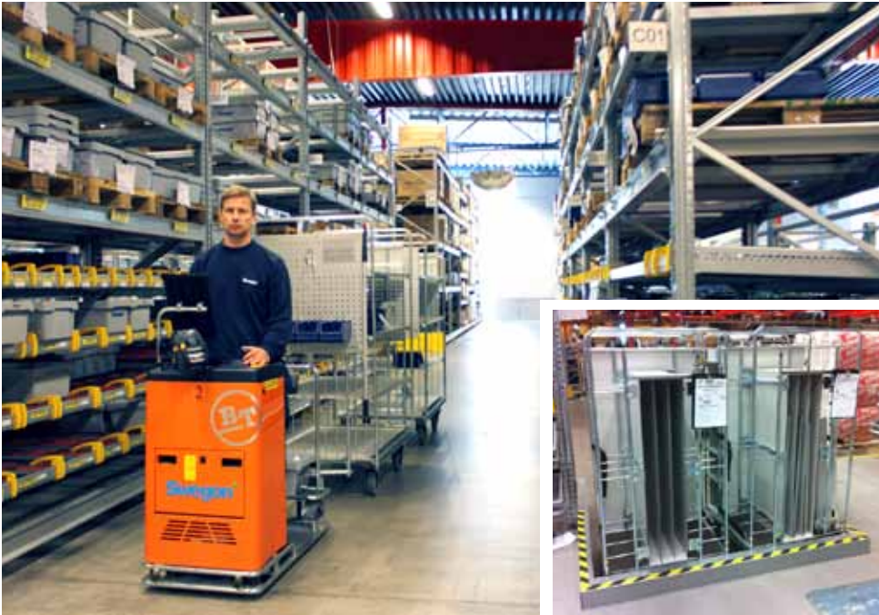
At Swegon AB they not only use ergonomic kit solutions, they also using refills trolleys in a so-called milk run to supply the technicians with materials and kept available. The trucks at Swegon AB were sold through Helge Nyberg AB's global partner Toyota Material Handling, under the brand name BT Movit.
