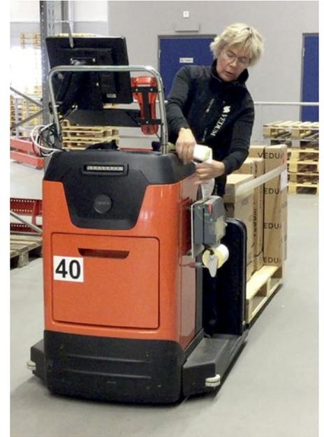
The label printer is located on the side of the forklift or on the backrest.
