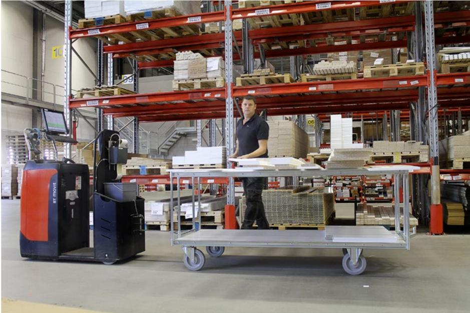
The trolley that is connected to the towing tractor is extra large to accommodate the long kitchen details.
