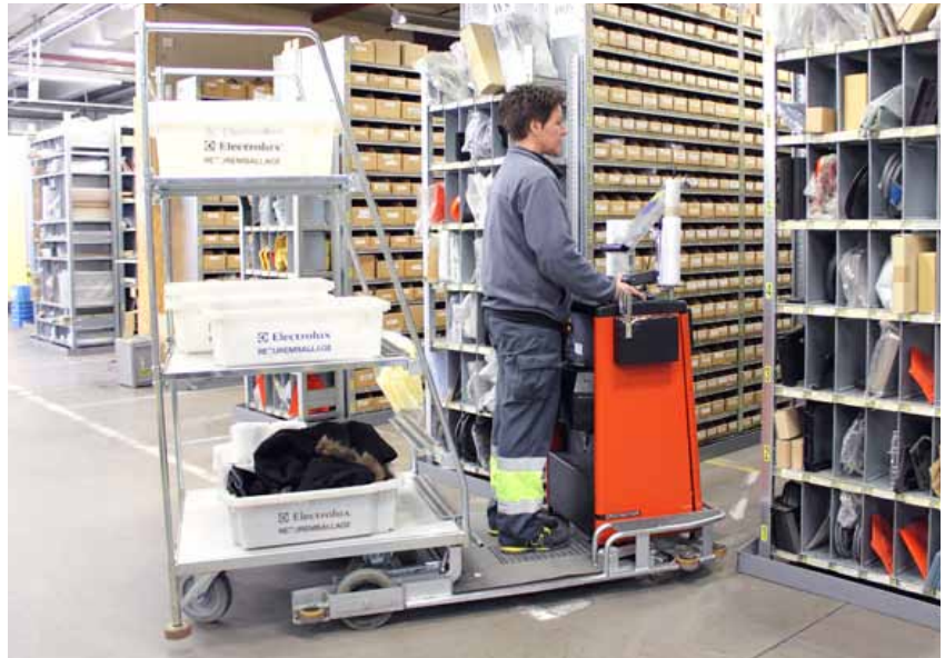
Guide rails in the floor simplifies the truck operator’s work when picking. The 2,8 meter picking height is easily reached using the steps.
