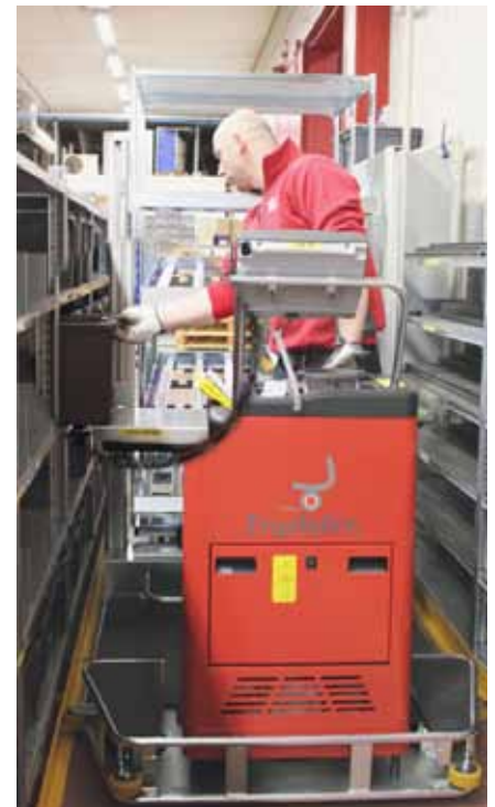
An automatic lifting table on the truck facilitates the work with material replenishment.
